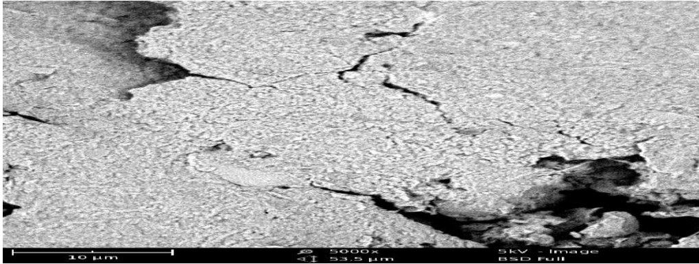
Plate 4.1b: Micrograph of black cotton soil optimally stabilized with 8 %lime / 8 % iron ore tailing blend after 7 days curing at 10 \mu\text{m} magnification
