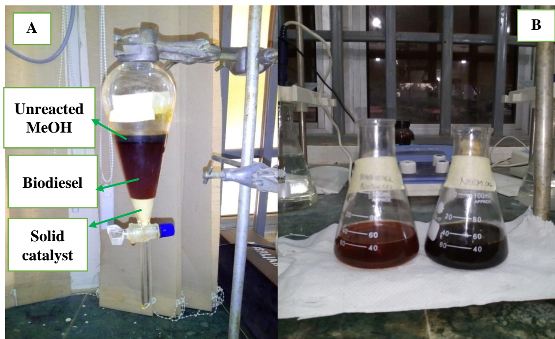
Plate V: a) freshly prepared neem oil biodiesel under separation b) decanted biodiesel and fresh neem oil
