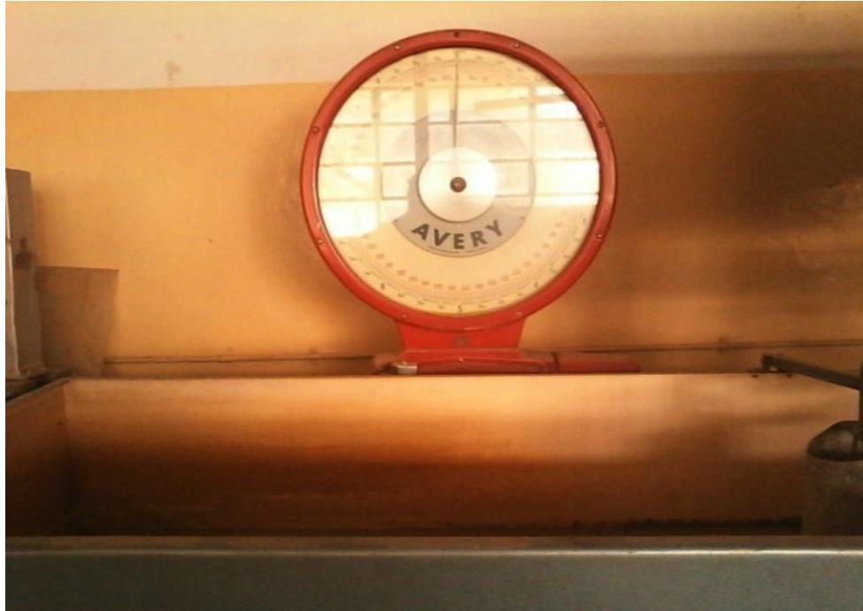
Plate 3.2 Pictorial view of weighing scale for measuring the discharge
