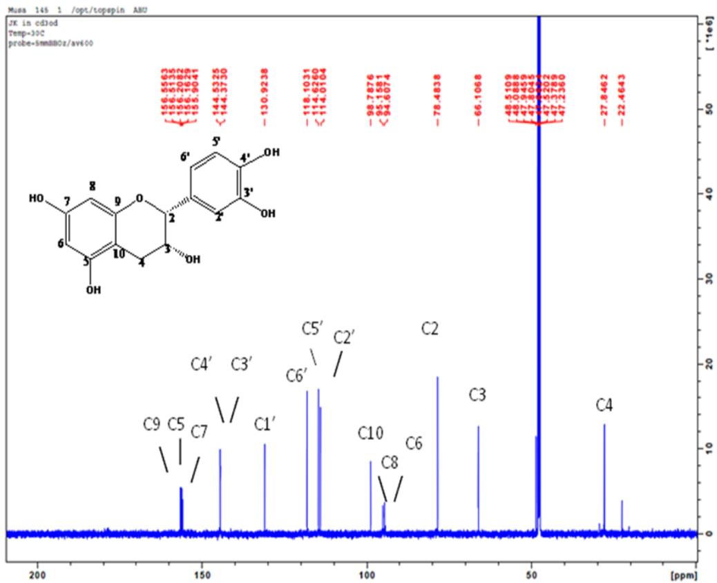
Fig. 4.2: <sup>13</sup>C NMR spectra of X1
