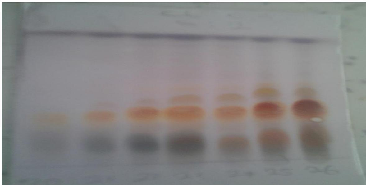
Plate 3: TLC profile of fraction 20 - 21 (Chloroform:Ethylacetate 8 : 2)
