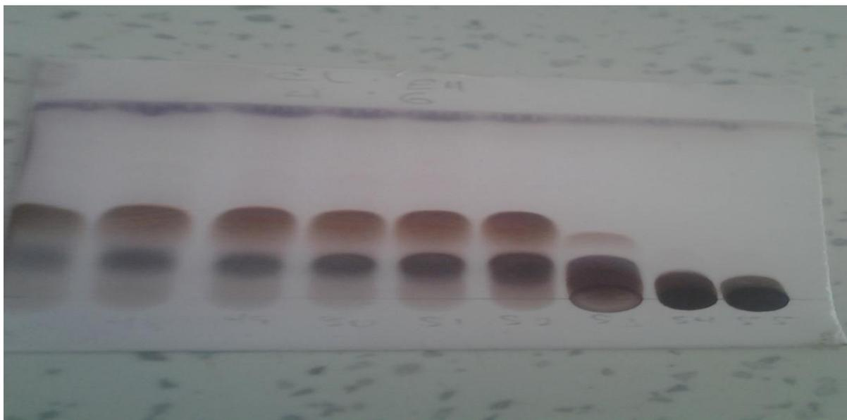
Plate 5: TLC profile of fraction47 - 55 (Chloroform:Ethylacetate 4 : 6)
