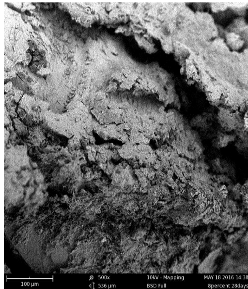
Plate IV: Micrograph of black cotton soil - 8% palm kernel shell ash mixture cured for 28 days at magnification of x500 (BSL compaction)
