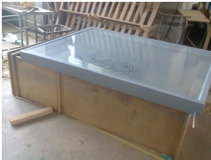
Plate 4: Finished solar collector with double galzing.
