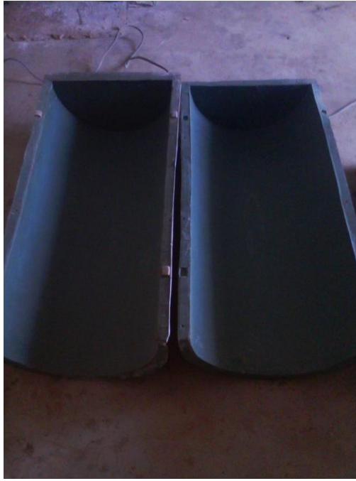
Plate5: Two halves of the hot water storage tank moulded using fibre glass and chemical binders
