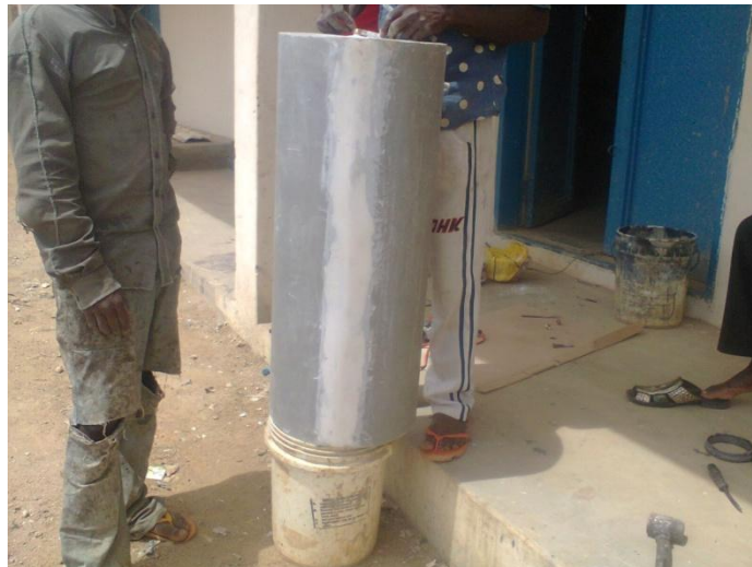
Plate6: The two halves of the storage tank joint together to form the complete hot water storage tank.
