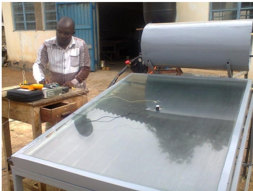
Plate12: System with experimental set up to measure system performance.
