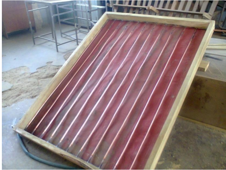
Plate3: Copper grid and absorber plate fitted into the collector casing
