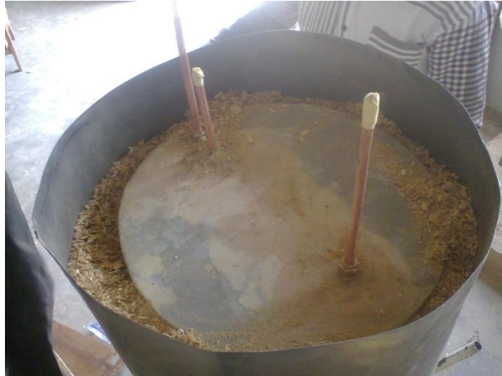
Plate7: The hot water storage tank inside a metallic cylinder rimmed with saw dust to prevent heat lost.
