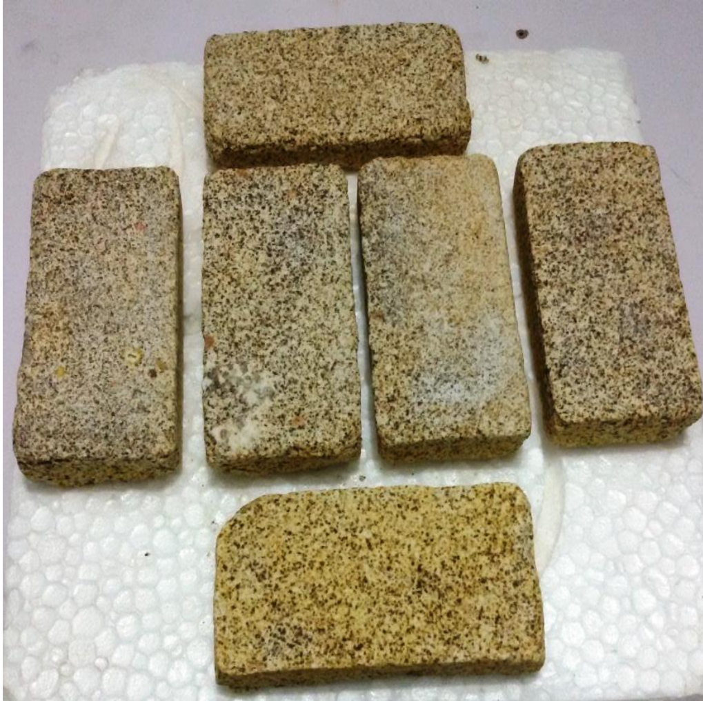
Plate 4.1 Surface Appearance of the Refractory Brick after Firing at 1450°C
