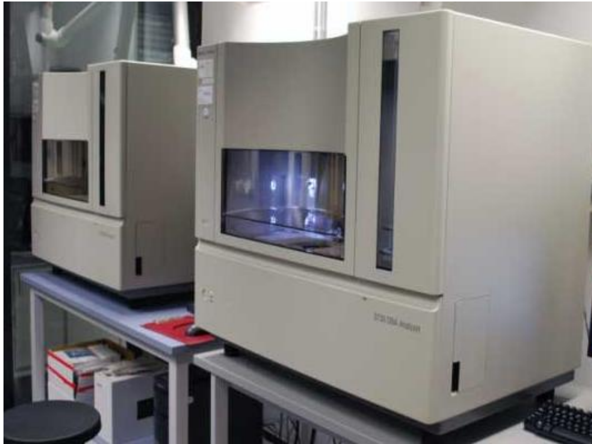
Figure 3.6: ABI® PRISM™ 3730 Genetic Analyzer (Applied Biosystems Foster City, CA). This 48-capillary tube analyzer is used for DNA fragment analysis and traditional DNA sequencing.
