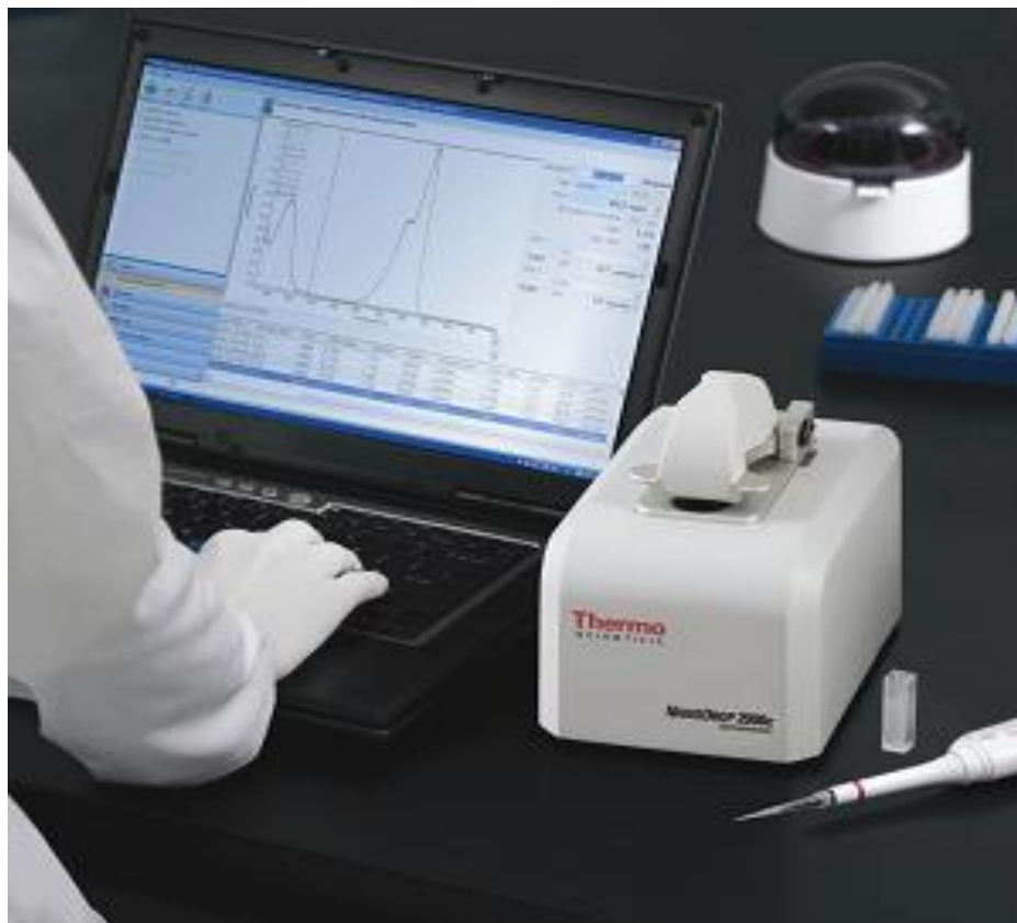
Figure 3.3: Quantitation of DNA. Using photo-spectrophotometry and absorbance curves to determine the quantity and quality of DNA with the NanoDrop™ 2000c (Thermo Scientific).
