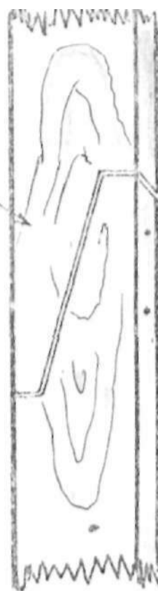
INCORRECT SPLICES IN TIMBER MEMBERS
