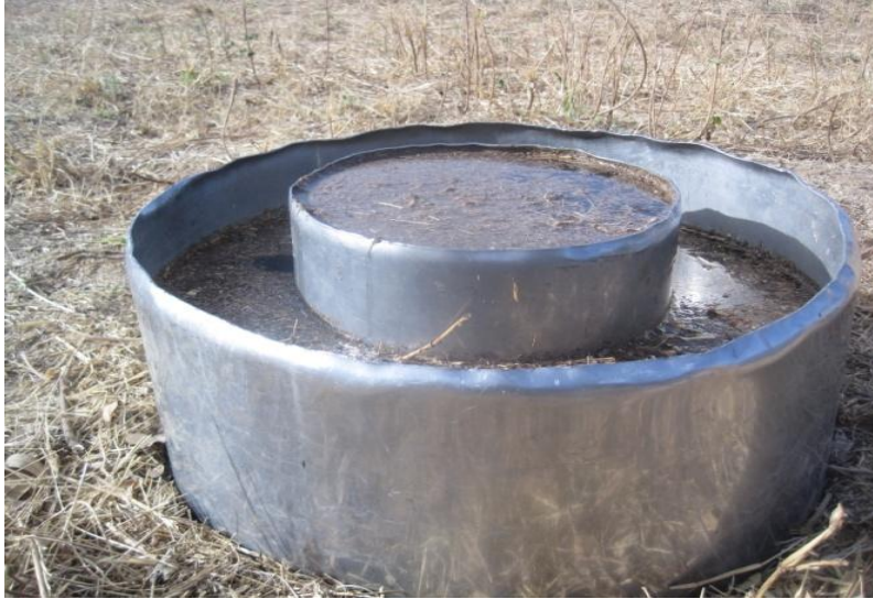
Plate 2.1: A set up of double ring infiltrometer ponded with water used in this study.
