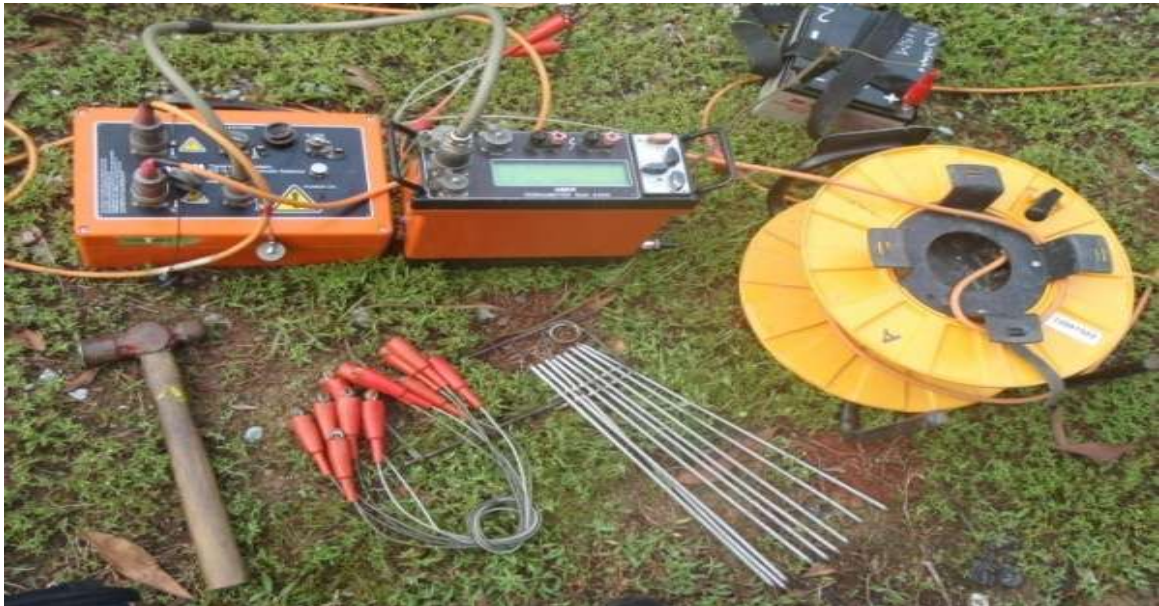
Plate 3.1: ABEM LUND Imaging system together with Terrameter SAS 4000 and ES 464.
