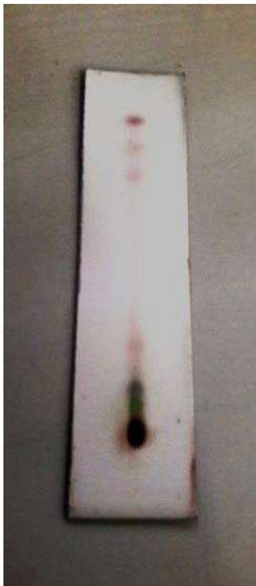
Plate III: TLC profile of n-butanol fraction ( \text{CHCl}_3 : MEOH; 9:1; 10% \text{H}_2\text{SO}_4 spray reagent)
