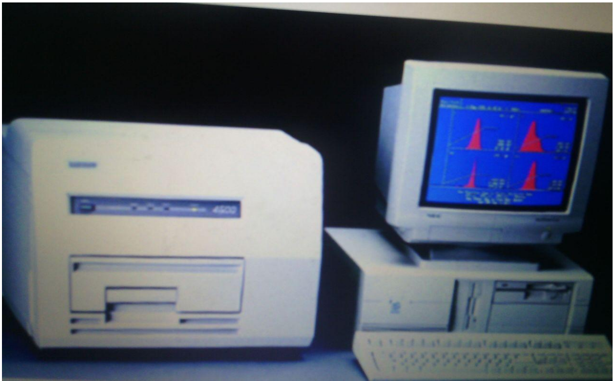
Plate 3. 1: Experimental set-up of Harshaw TLD Reader and PMT
