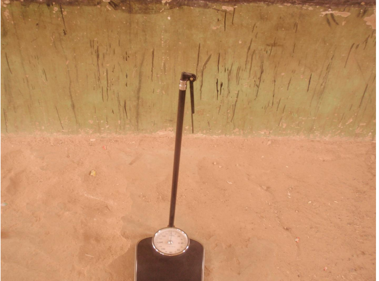
Plate IV: Stadiometer used for the measurement of height and weight
