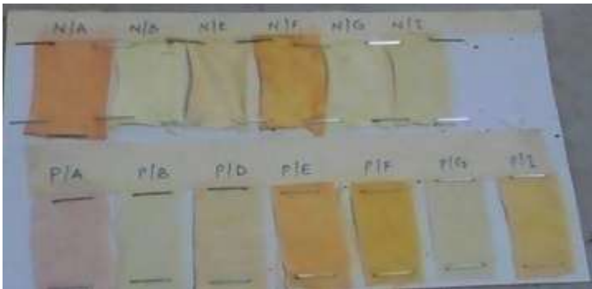
Plate III: Dyed samples (N – Nylon 6; P – Polyester)
