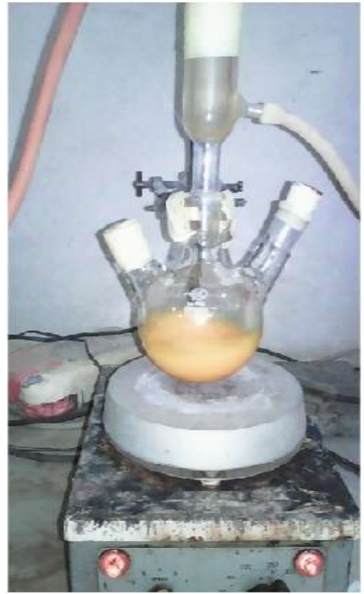
Plate II: Synthesis setup for Dye B
