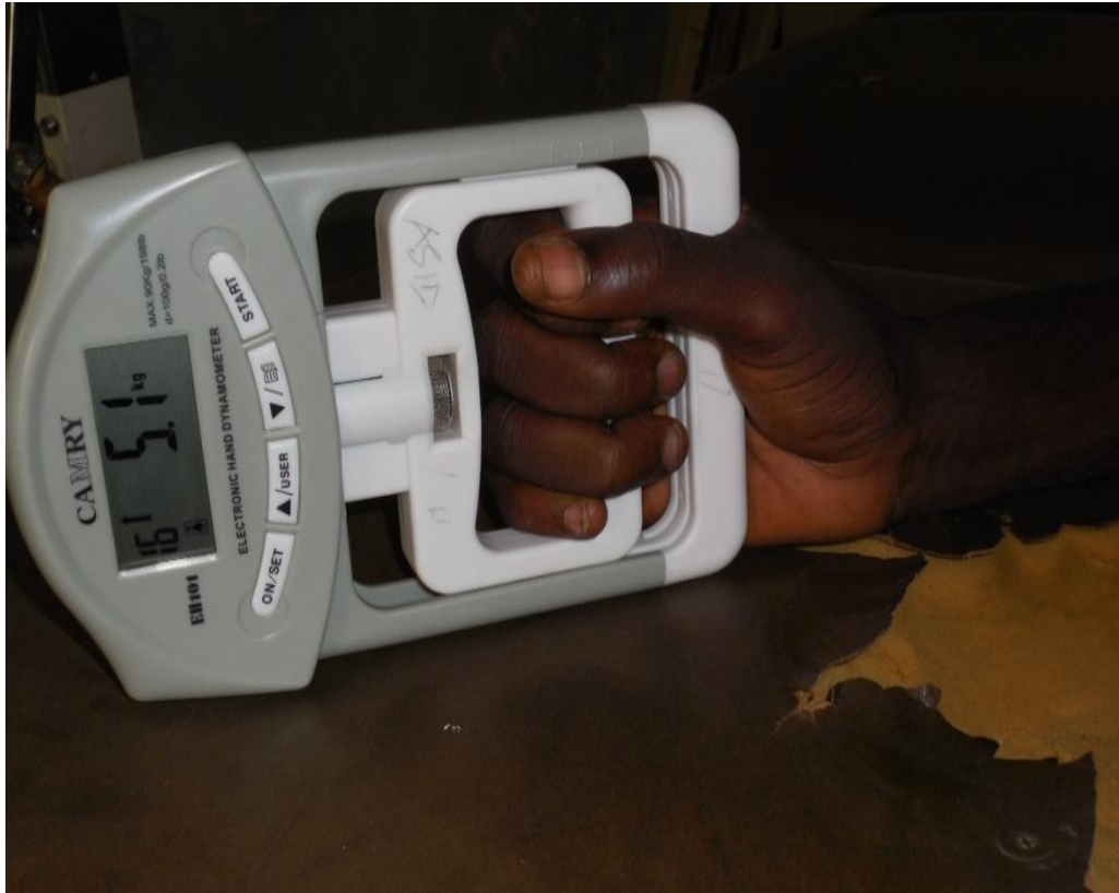
Plate V: Camry digital hand-grip dynamometer for measuring hand-grip strength
