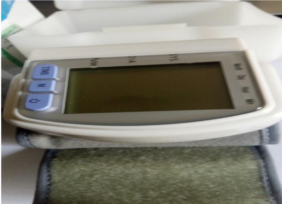
Plate X: Digital sphygmomanometer for measuring blood pressure and pulse rate
