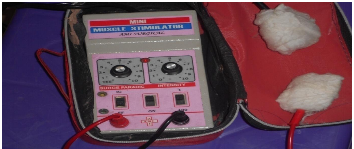
Plate 1: Mini-electrical stimulator for stimulation of muscle (Ami Surgical, 13ko1126c, Mumbai, 2003).
