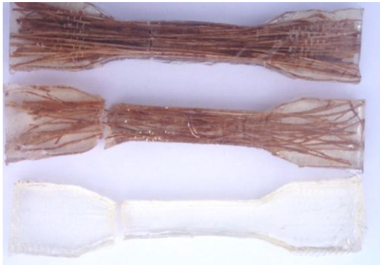
Plate III: Fractured tensile test samples
