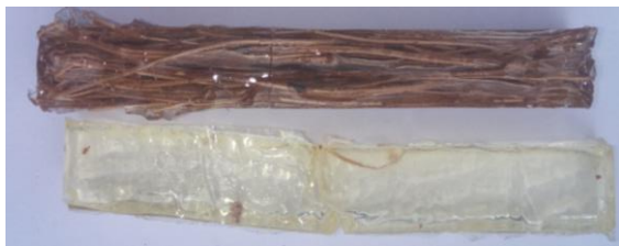
Plate IV: Ruptured flexural test samples
