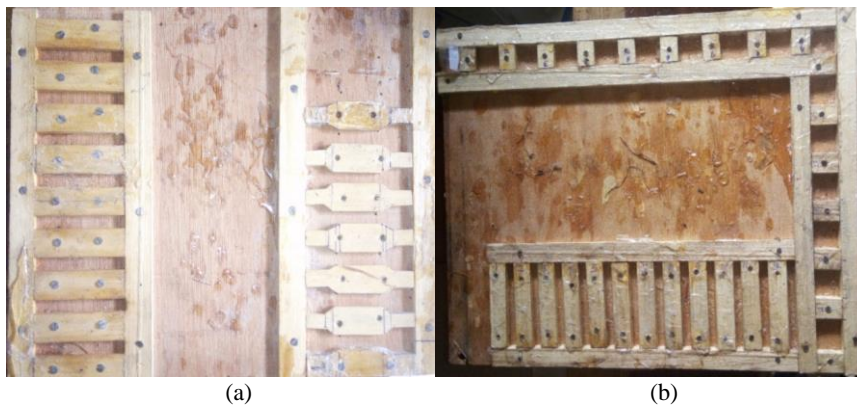
Plate II: Wooden moulds (a) for DMA and tensile test samples; (b) for hardness and flexural test samples
