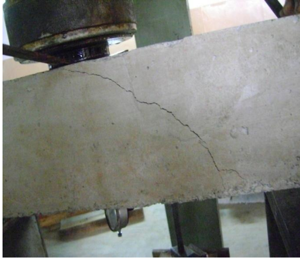
Appendix A-14: Failed beam specimens
