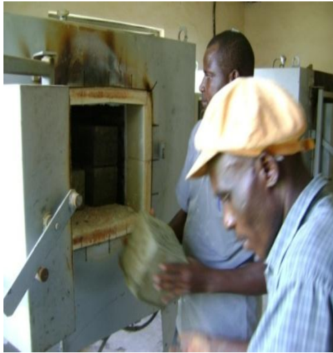
Plate x: Loading of specimens in to heating chamber (electric furnace)
