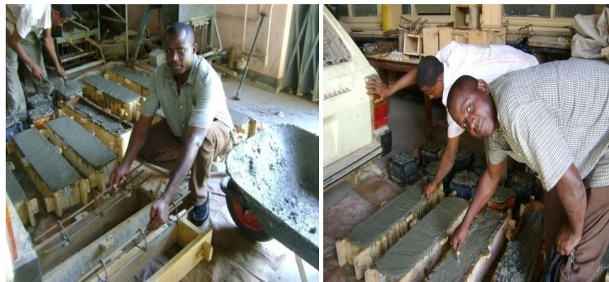
Plate VIII: Preparation of test Specimens ( Prisms)
