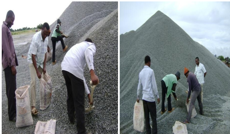
Plate VII: Sourcing of Coarse aggregates (20mm, 14mm and 10mm) at Mother
