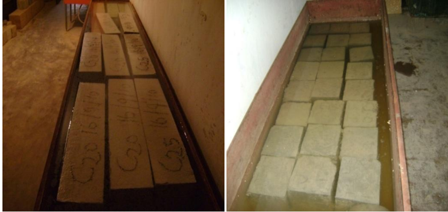
Plate IX: Curing of Concrete Specimens
