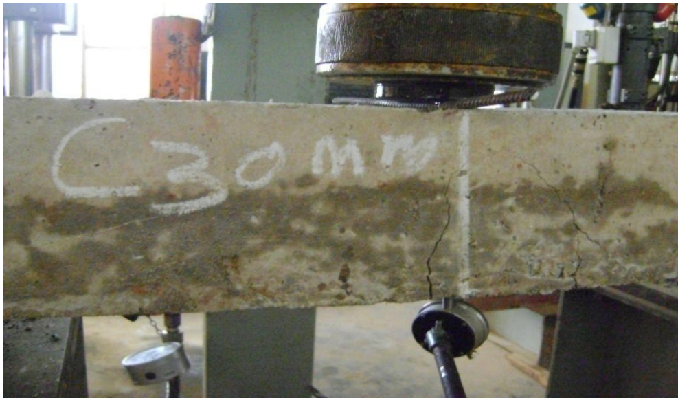
Plate xii: Three Point Bending Test in progress with crack propagation on specimen's surface
