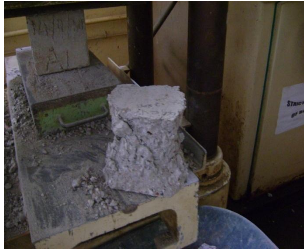
Appendix A-15: Failed cube specimens
