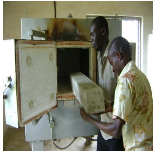
Plate x: Loading of specimens in to heating chamber (electric furnace)
