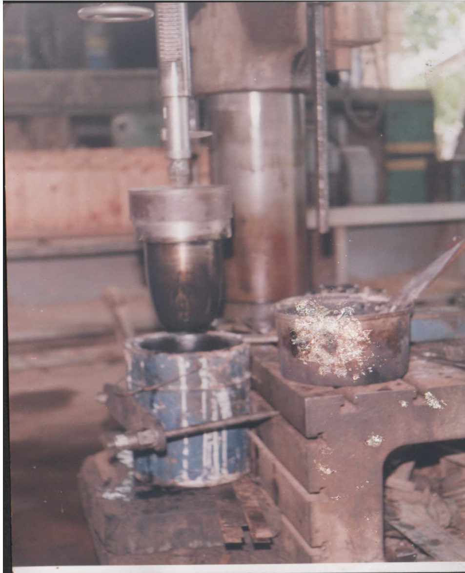
Plate 3.7: Setting of the Female and Male Moulds Prior to Pressing.
