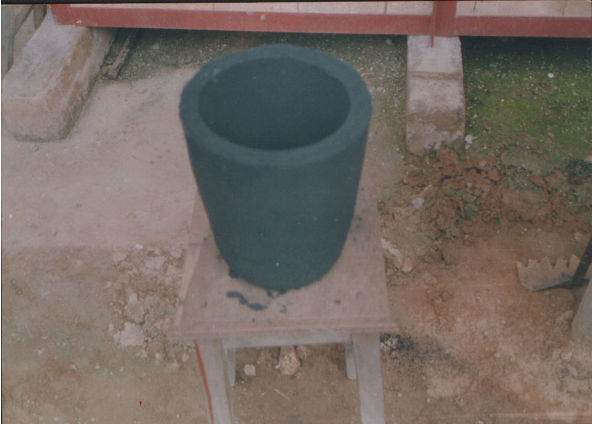
Plate 3.9: The Green Crucible Produced
