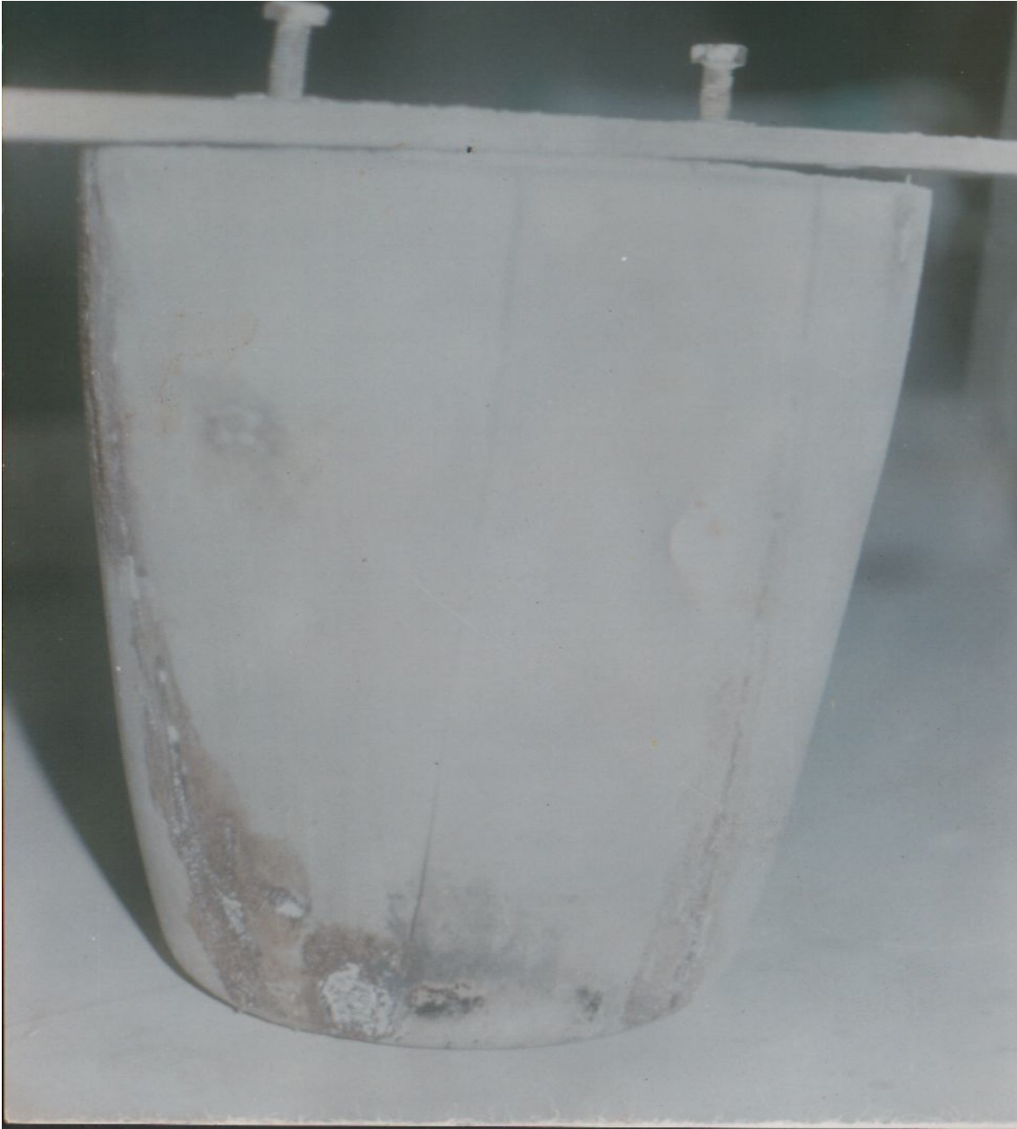
Plate 3.2: The Wooden Pattern Used for Producing the Female Mould.
