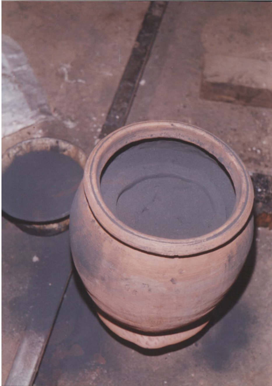
Plate 3.10: Preparation of the Crucible for Firing
