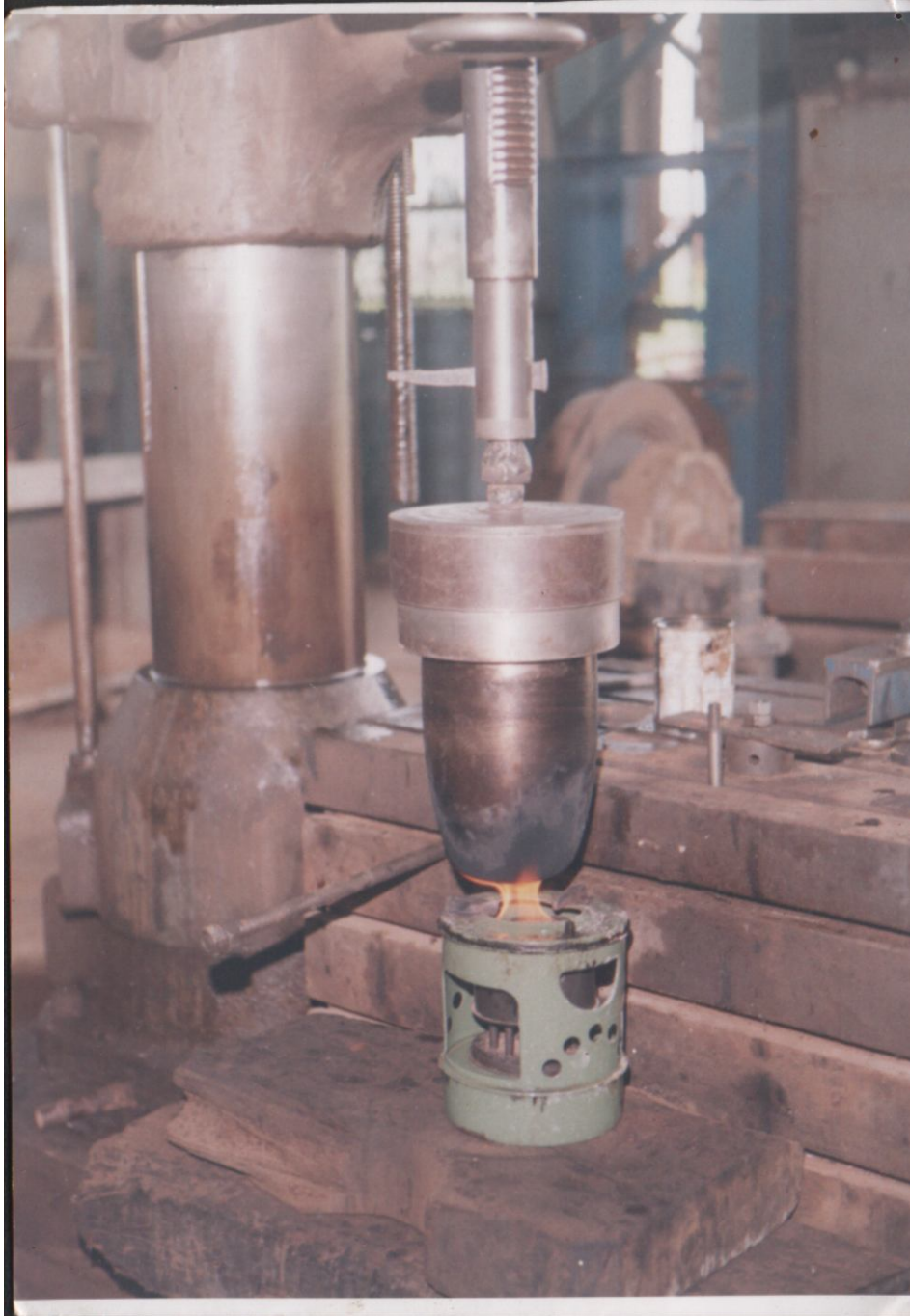
Plate 3.6: Heating of the Male Mould.
