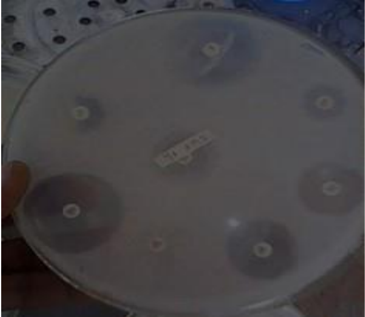
Appendix I: Antibiotic susceptibility test on Mueller Hinton agar using Kirby-Bauer disc diffusion technique.
