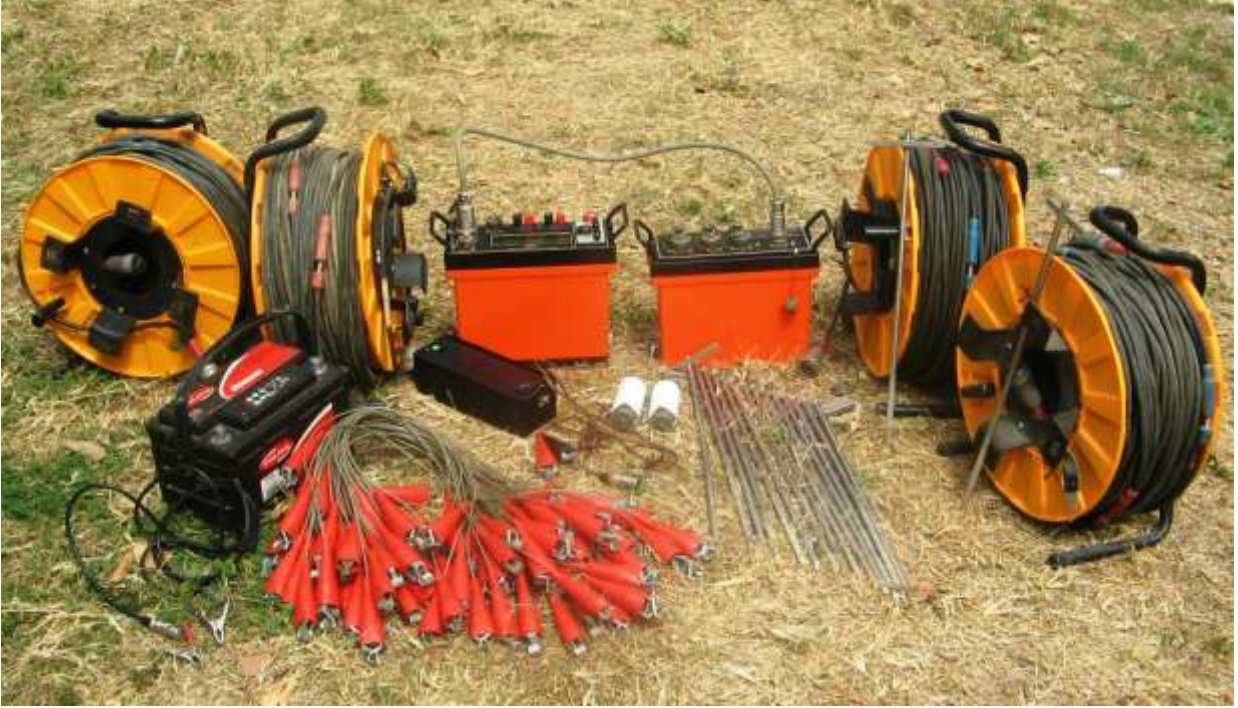
Plate II: ABEM LUND Imaging system together with Terrameter SAS 4000 and ES 464.
