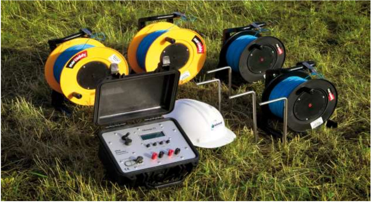
Plate III: OHMEGA \Omega Resistivity meter with its accessories
