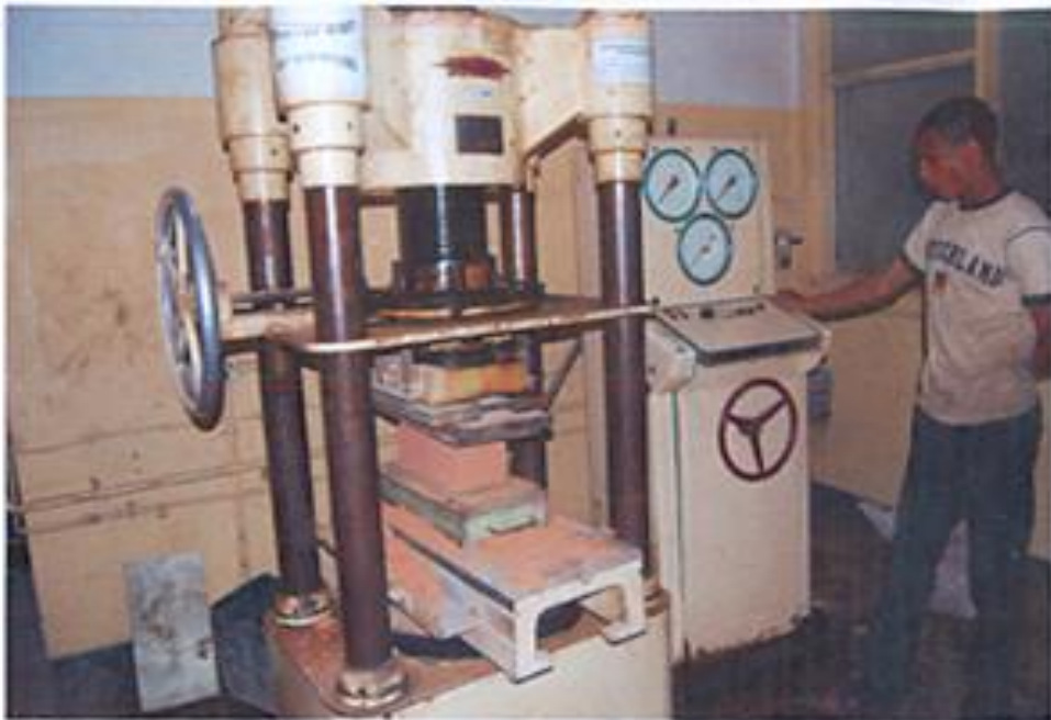
Plate 6: Crushing of blocks for compressive strength test
