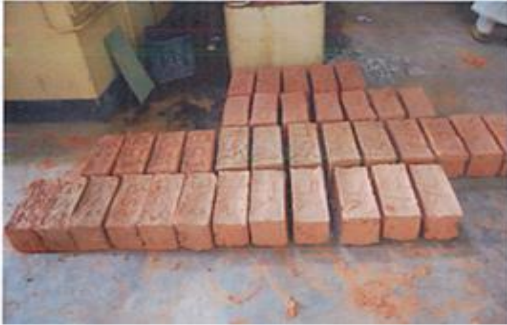
Plate 5: Blocks ready for compressive strength test
