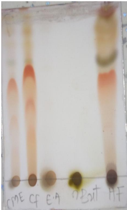
Plate II: TLC profile of CME, HF, CF, EF and BF in hexane-ethyl acetate (5:3).
