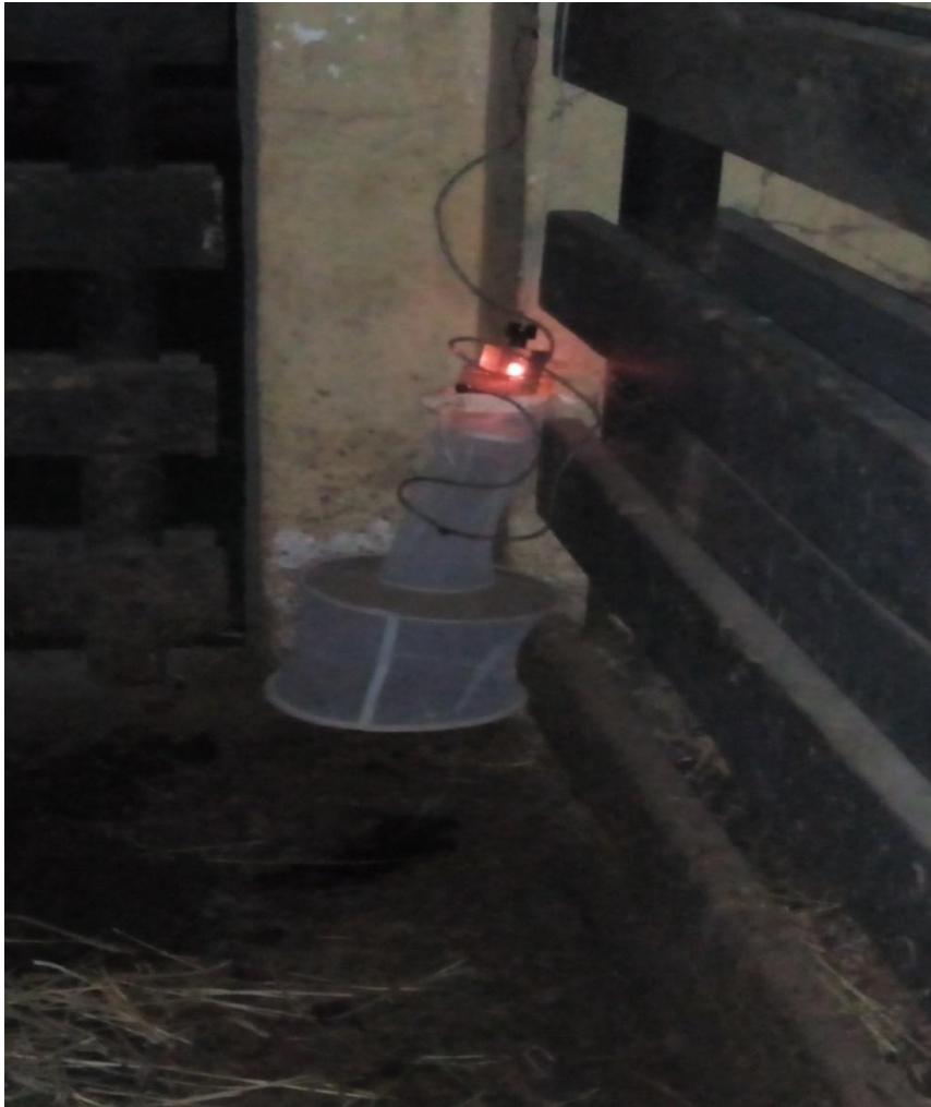
Plate IV: Center for Disease Prevention and Control (CDC) miniature light trap for mosquitoes collection.
