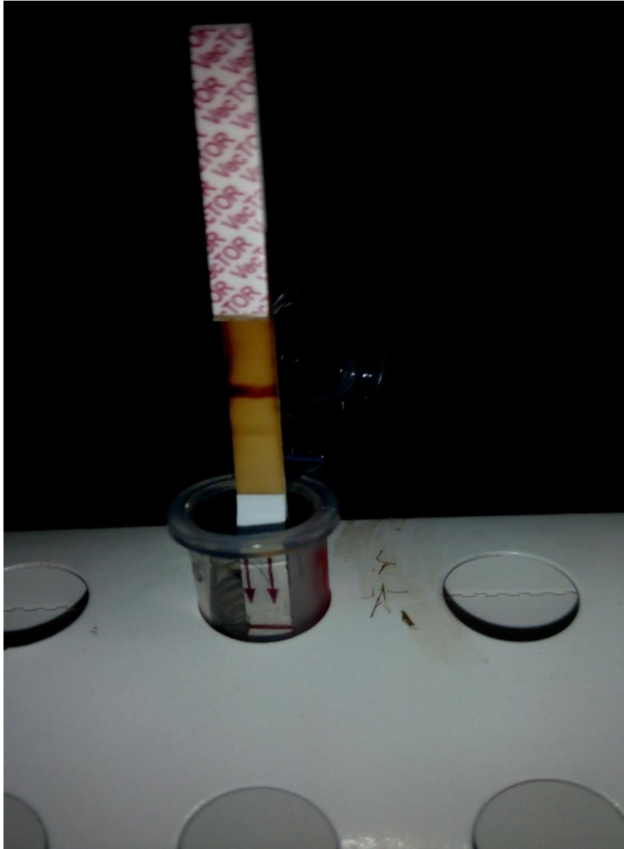
Plate III: A VectorTest (R) dip stick for a positive pool of mosquitoes. The second band below the control band is an indication of positive result for presence of WNV antigen in mosquito pool.
