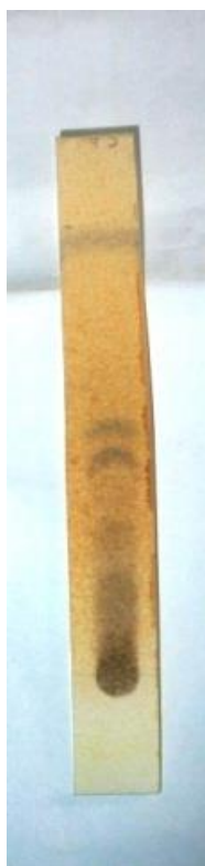
PLATE VIII: Thin Layer Chromatogram of Aqueous Methanol Leaf Extract of D. arborea after Spraying with Ferric Chloride Spray.
