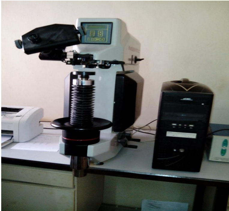
Plate; II: Identec universal hardness testing machine type 8187.5 LKV model B (ABU, Zaria)
