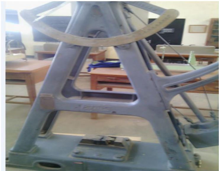
Plate; I: Izod impact testing machine used for the impact test.
