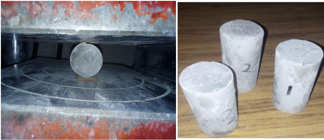
Plate XIII: RPC samples under tensile strength test
