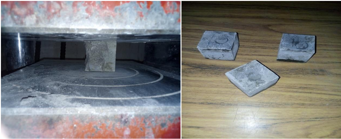
Plate XII: RPC samples under compressive strength test
