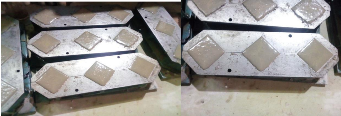
Plate X: Sample of RPC after casting
