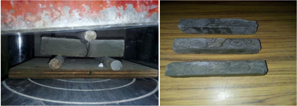
Plate XIV: RPC samples under flexural strength test
