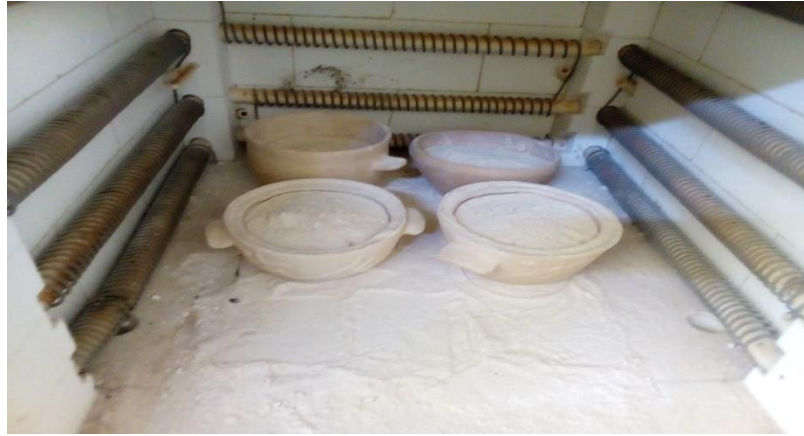
Plate VII: Furnance with kaolinite to be calcined
