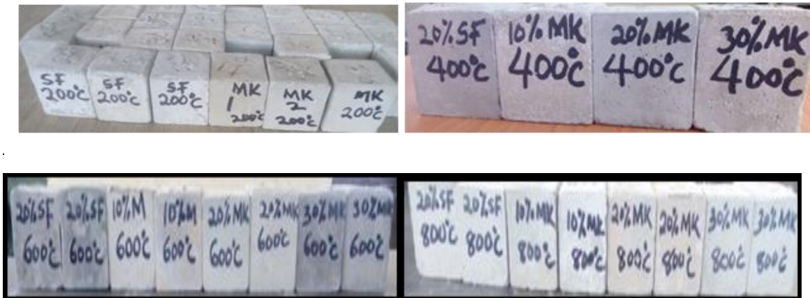
Plate XXI: Sample exposed to elevated temperatures
