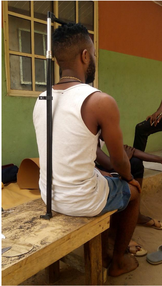
Plate VII: Measurement of sitting height (cm) using an anthropometer (Belo Horizonte, Brazil).
