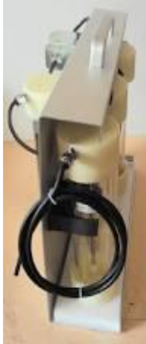
Plate III: Gas conditioning System
